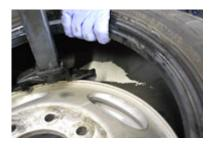
6) If using the Pour In method, this is what it should look like. Remember, it's extremely important to place the beads or the bag opposite the valve stem. If you don't, the air blast will blow the beads around and they may get stuck between the tyre bead and the rim.
