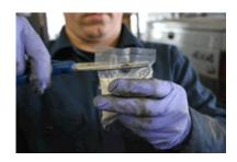
3) Using scissors, cut the seal off of the bag. You must do this whether you are using the Bag In tyre method or the Pour In method.
