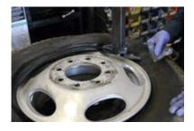
7) Install the top tyre bead onto the rim
