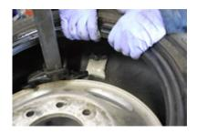
5) If using the Bag In tyre method, gently place the bag upright against the outer wall, and opposite the valve stem.
