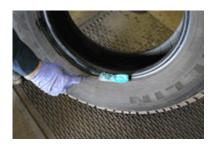
1) Carefully apply bead lube to the tyre in the area shown only using the method shown. DO NOT twirl the swab in a circle as most mechanics do. This will fling bead lube into the tyre. If any bead lube gets into the tyre, IT MUST be wiped out with water. Never coat the rim
